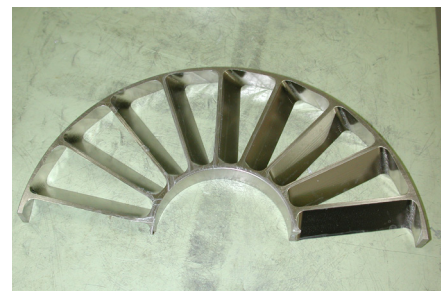
Figure 2: - Changing the shape of the leading edge of the upper rotor blades reduces the number of particles that rebound back into the process chamber (simulation results). A new rim on the stator blades reduces the accumulation of by-products.
